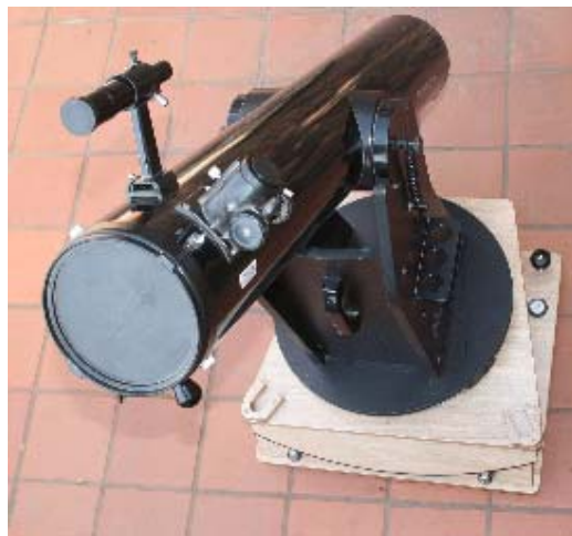
The Dobtorial platform provides one hour of equatorial tracking for Dobsonian telescopes.
